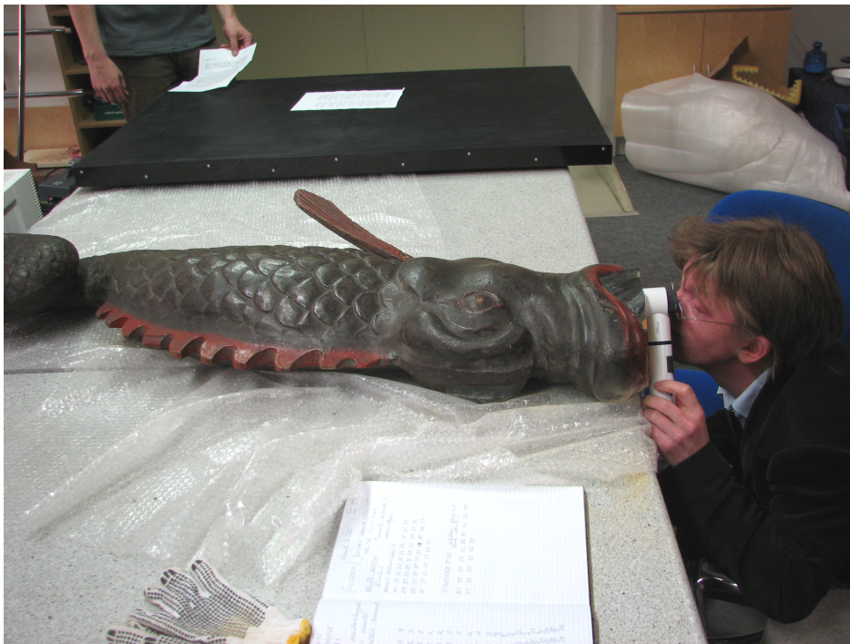
Figure 3. Ring widths were measured from the mouth of the whale to the nearest 0.1 mm by the Eschenbach 10× measuring lens
