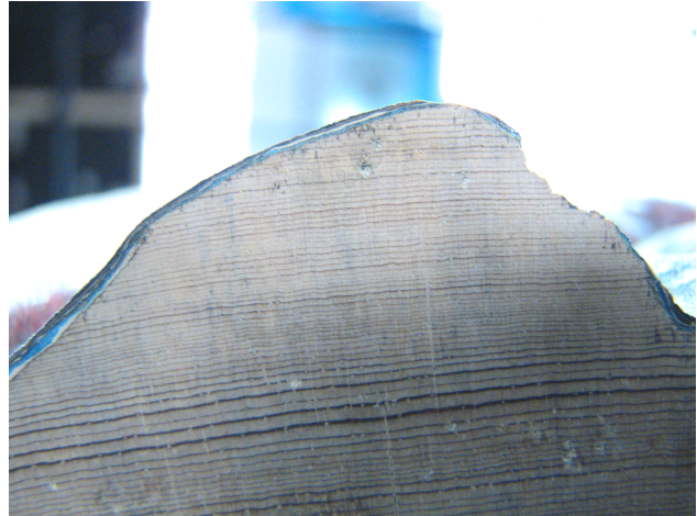
Figure 7. The outer surface of the cross section of the mouth of the whale at radius 2. The silhouette does not follow the ring borders
